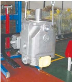
2.Hoist via cross holes of flange by double-hook
