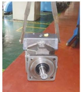
1.Hoist the pump via the ends of the bolts
